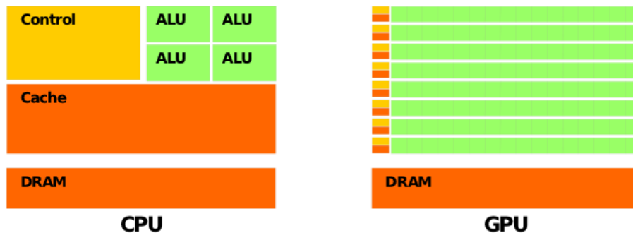
Figure 1: Differences in GPU and CPU hardware architecture
